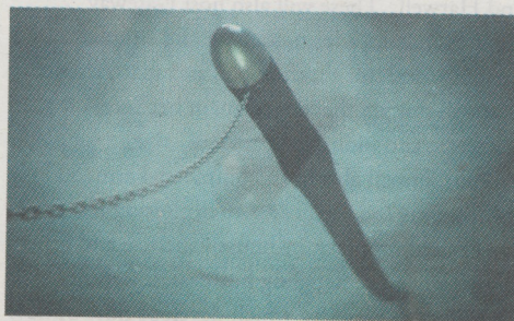
The Anaconda wave energy capture device, designed by Atkins'
